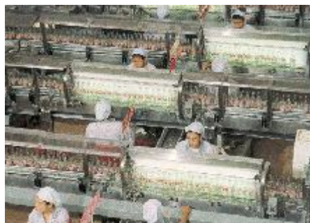
Visual Empty Bottle Inspection
