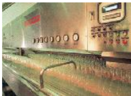
Washed Bottles Discharge Conveyo
