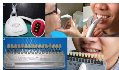
Figure 1 a-f. Showing the instrumental and visual color measurement for this study (a-c) using spectrophotometer (Vita Easyshade® Advance 4.0) (d-f) using shade tab (VITAPAN classical shade tab)
