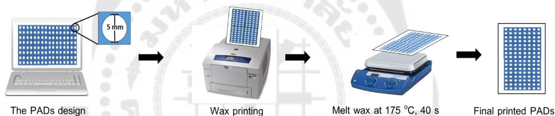
Figure 9 Design and fabrication of the PADs by wax printing method.
