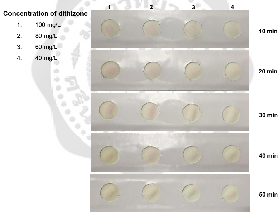
FIGURE 57 Effect of time shows the image of the colorimetric response after adding of Ag ion (100 \mu\text{M} ) into paper based with different dithizone concentration of 40 mg/L, 60 mg/L, 80 mg/L and 100 mg/L, respectively.
