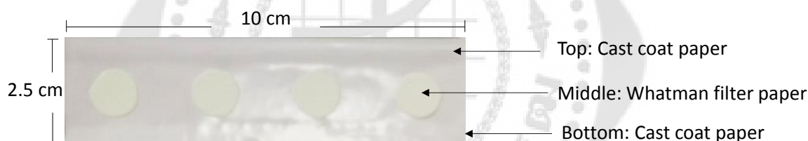
FIGURE 7 Design of the paper based device.
