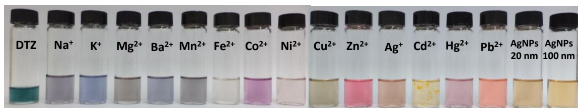
FIGURE 32 Visual color change of the other metal ions ( 1.951 \times 10^{-4} M) solution after addition of dithizone in ethanol with the concentrations of 10 mg/L.
