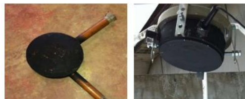
Fig. 2 Calorimeter made of copper and stainless steel (both areas 0.0154 \text{ m}^2 )
