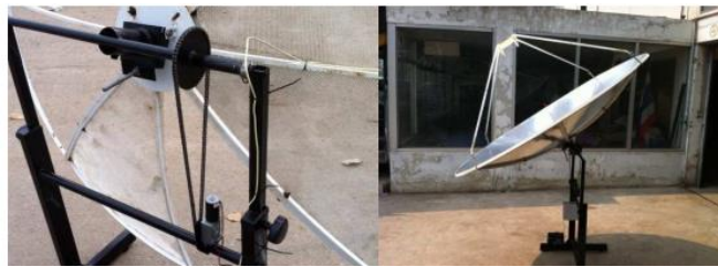
Fig. 1 A constructed parabolic dish collector with the electronic controlled sun tracking system.
