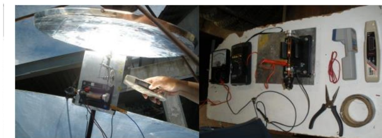
Figure 9 The apparatus arrangement for an engine-generator output experiment.
