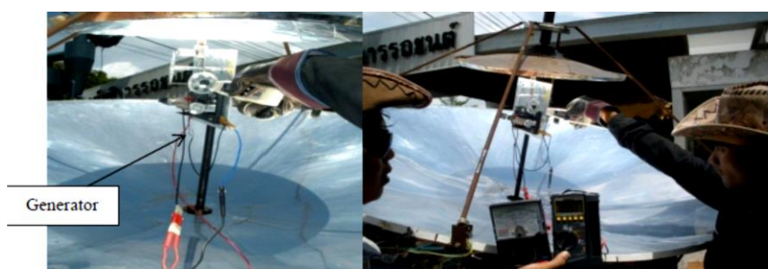
Figure 10 The measuring instrument for engine-generator output experiment.
