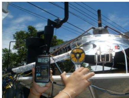
Figure 6: Aphotograph of calorimeter and thermocouples.
