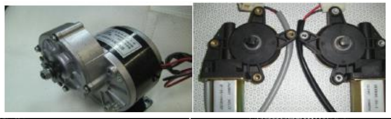
Figure 11: A 24VDC 250 W motor with gear ratio 1:5 at 600 RPM for elevation movement and a 12 VDC wiper motor 110 RPM for azimuth movement.
