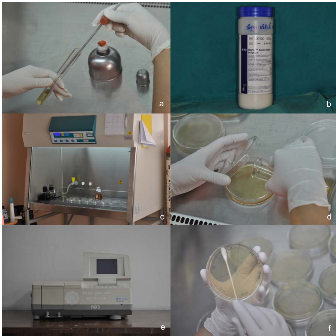
Figure 11 Preparation of bacterial suspension and BHI a) Cultivation of S. mutans b) BHI powder c) Laminar flow hood d) Preparation BHI agar e) UV-spectrophotometer f) S. mutans spread on BHI agar.
