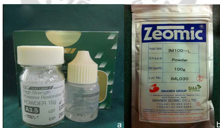
Figure 6 Materials used in this experiment. a) Highly viscous glass ionomer cement (Fuji IX TM GP) provided as powder and liquid system. b) SZ (Zeomic ® ) as white powder
