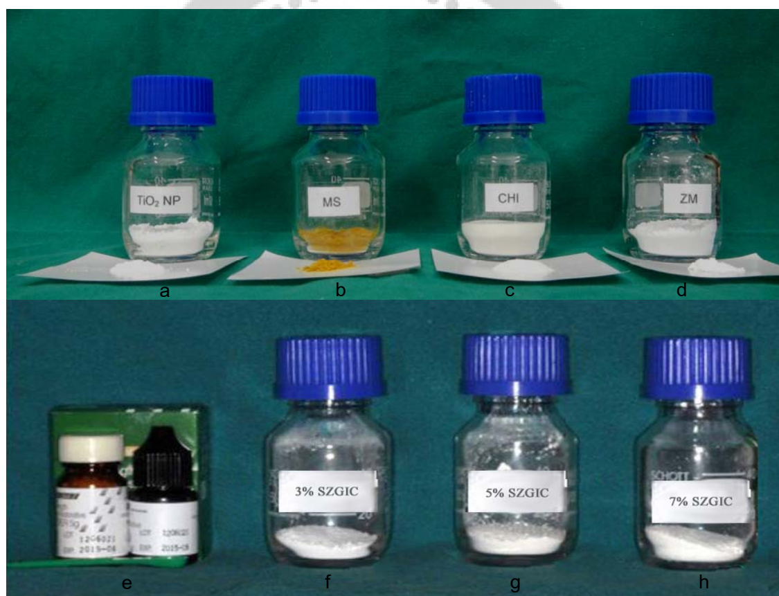
Figure 9 Materials used in this study a) Titanium dioxide b) Extract from pericarp of mangosteen c) chitosan c) SZ e) Conventional glass ionomer cement powder (Fuji IX TM GP) f), g), h) Conventional glass ionomer cement powder mixed with SZ (Zeomic ® ) at 3.0%, 5.0%, and 7.0%.
