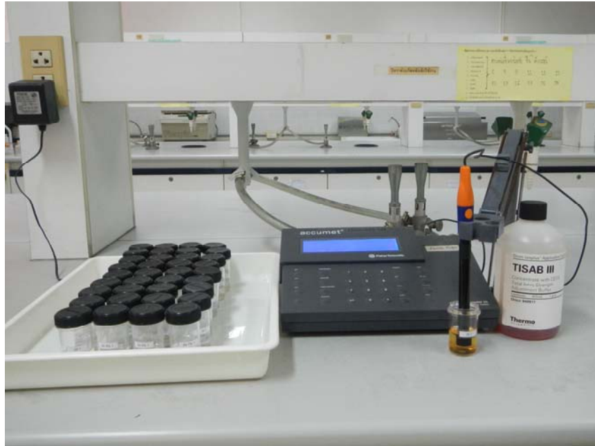
Figure 23 Disc-shaped specimens in deionized water. De-ionized water 5 mL and buffer solution (TISAB III) 0.5 mL were measured for the fluoride release.
