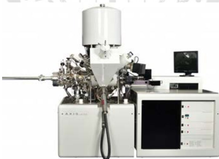
Figure 39 AXIS Ultra DLD (Kratos Analytic Ltd.), XPS
