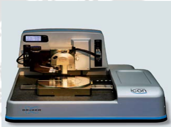
Figure 34 Bruker's Dimension Icon® Atomic Force Microscope (AFM) System using for measuring the surface roughness of thin films.
