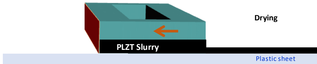
Figure 14 Model of hand tape casting of PLZT
