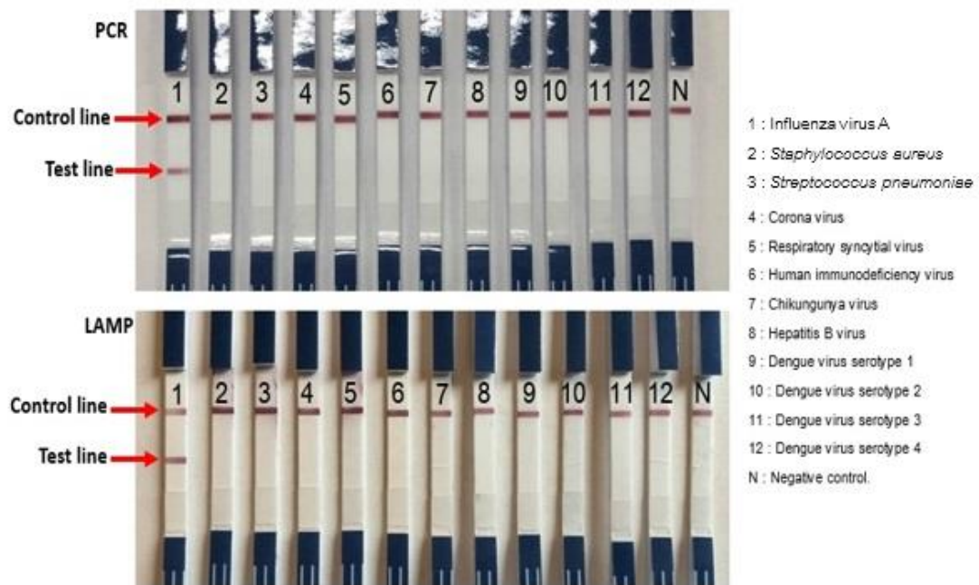
Figure 26 Specificity test of PCR-LFD and LAMP-LFD assays. Strips 1-8 represents S.aureus , S.pneumoniae , Corona virus, Respiratory syncytial virus, Human immunodeficiency virus, Chikungunya virus, Hepatitis B virus, Dengue virus serotype 1-4, respectively. Strip N represent negative control.
