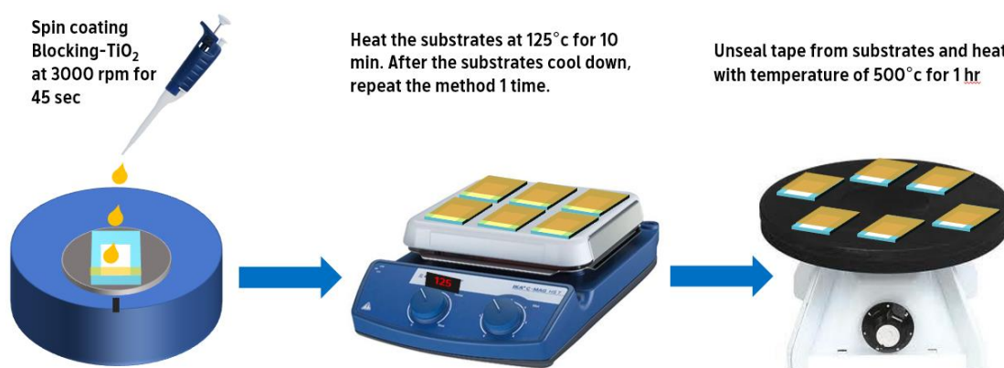
Figure 30 The summary of blocking layer preparation process.
