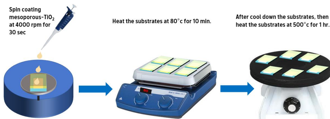
Figure 31 The summary of mesoporous-TiO 2 deposition method
