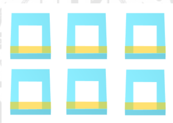
Figure 29 the FTO glass attached by capton tape.
