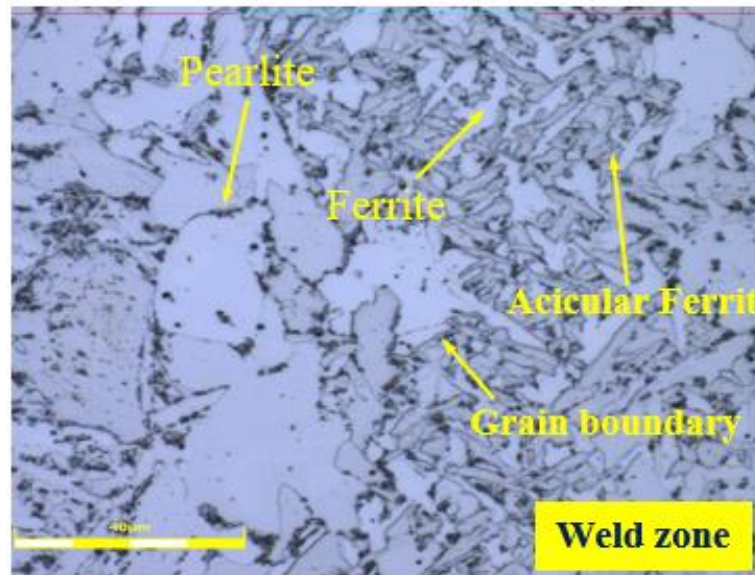
Figure 66 Variety of grain sizes at Welding zone (EH36 & EH36)
