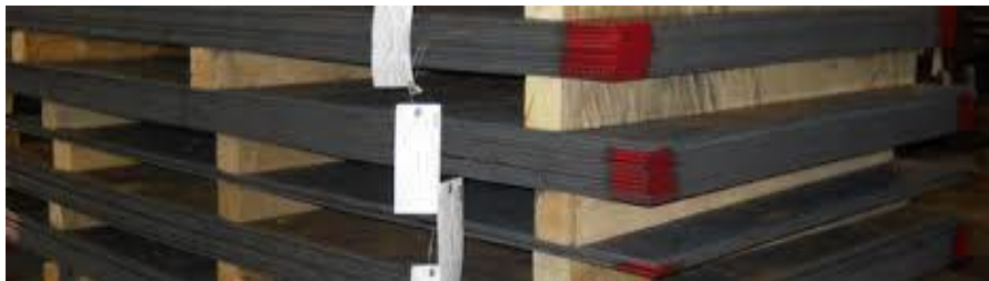
Figure 42 HSLA Steel (ABS EH36)
