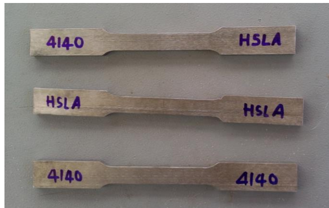
Figure 50 Specimens shape for tensile testing (Welding joint)
