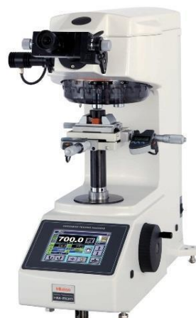
Figure 51 Micro-Vickers hardness testing machines (MITUTOYO: HM-210A)
