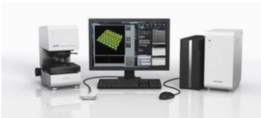
Figure 54 Optical microscope (Olympus laser microscopes model OLS 4000)
