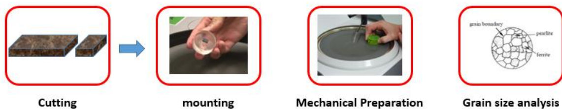
Figure 52 Metallography examination process
