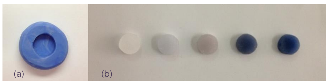
Fig 2 mould(a) and specimen(b) for antimicrobial activity test : Disc-shaped specimen
