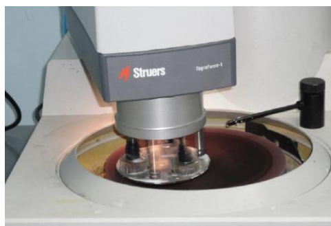
Figure 29 Polishing of the specimen with rotary discs.
