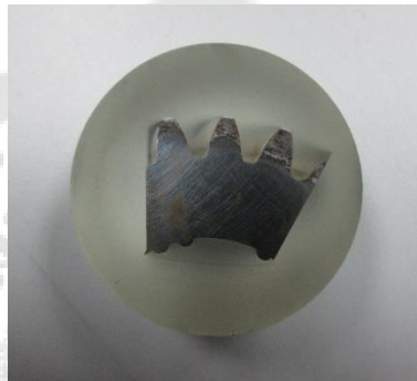
Figure 28 Mounting small a sample specimens in a synthetic resin.
