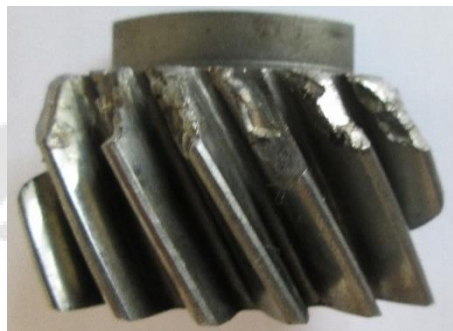
Figure 32 A sample specimen of the fracture surface cutting from the pinion gear.
