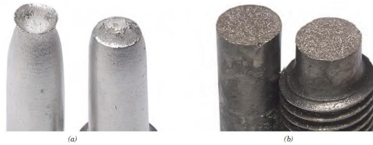
Figure 5 (a) Cup-and-cone fracture in aluminum. (b) Brittle fracture in a mild steel. (From William D. Callister, Jr., Materials Science and Engineering an Introduction Failure , Seventh edition, Copyright 2007 by John Wiley & Sons, Inc.)
