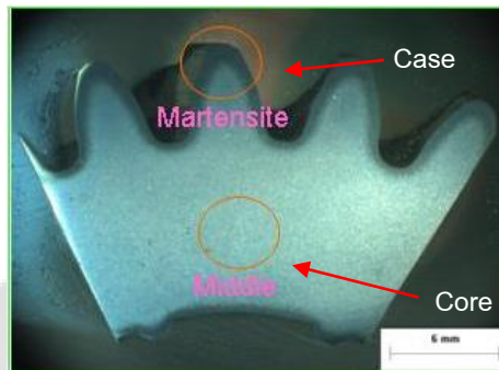
Figure 30 A sample specimen look through an optical microscopes at the outer surface and the central region.
