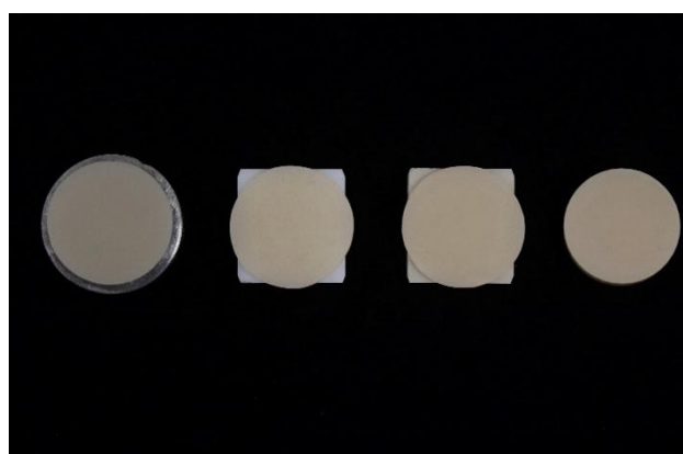
Figure 1 The 1 mm-thick zirconia specimen on titanium, white zirconia, and yellow zirconia backgrounds and control specimen (from left to right)
